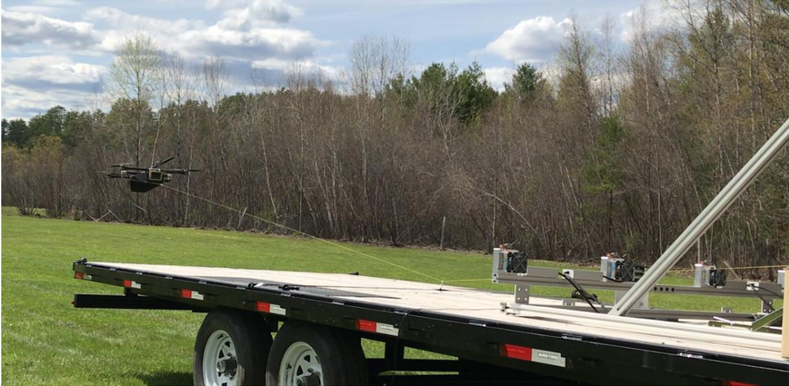
Figure 5-13: Outdoor testing setup for the air wake measurement system. Pictured are the trailer bed, meant to stand in for a ship deck, with mounted IR beacons, the tether reel controller, and a base station GPS. The UAS platform is seen engaged in tethered flight as the tether line is doled out to its specified sweep length.
