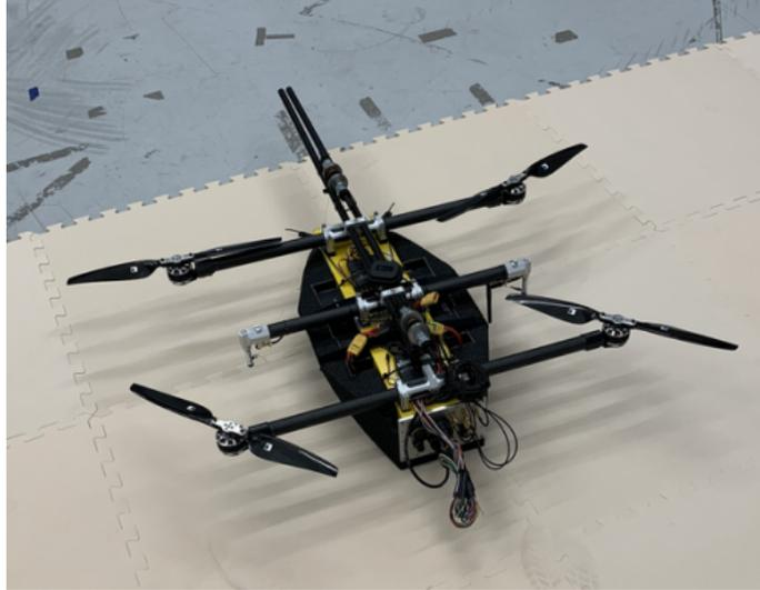
Figure 3-3: Outdoor flight testing platform for the air wake measurement system. An air probe placeholder is shown extending out of the front of the airframe, and the tether attachment points protrude out of the airframe's sides. The yellow housing, which contains all onboard computers and all sensors except for the GPS antenna and air probe, is surrounded by a black foam casing for protection.
