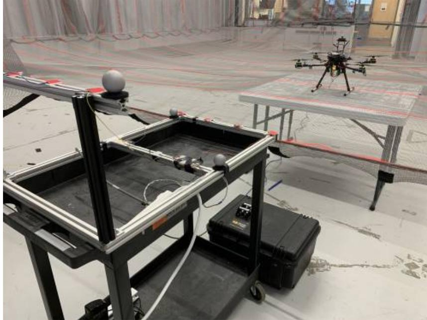
Figure 3-2: Indoor flight testing platform for the air wake measurement system, pictured within the Vicon motion capture space used to spoof GPS sensing.
